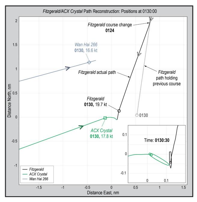
Figure 10. NTSB path reconstruction for *Fitzgerald* and *ACX Crystal*, from data compiled from NTSB Vehicle Performance Study.
