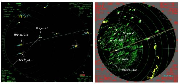
**Figure 6.** A comparison of radar screens from different vessels before the collision. Left, screen capture from the *Wan Hai 266* electronic navigation software, about 6 minutes before the collision. Right, screen capture from the *ACX Crystal* electronic navigation software (radar and ARPA), at the same time. (Vessel names have been added to screen images.)
